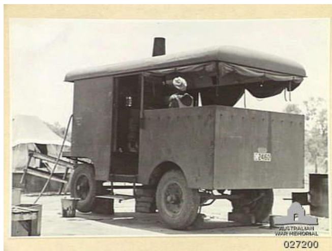
Cooker Number 17, an early production Wiles Cooker in use with 119 Australian General Hospital at Adelaide River, Northern Territory, in October 1942. This one was manufactured under Contract Demand E7126 issued on 23 October 1941. Note the rounded wheel arches and platform at the front. This is fitted with a fixed roof with a sliding hatch. (AWM 027200 – copyright expired)
