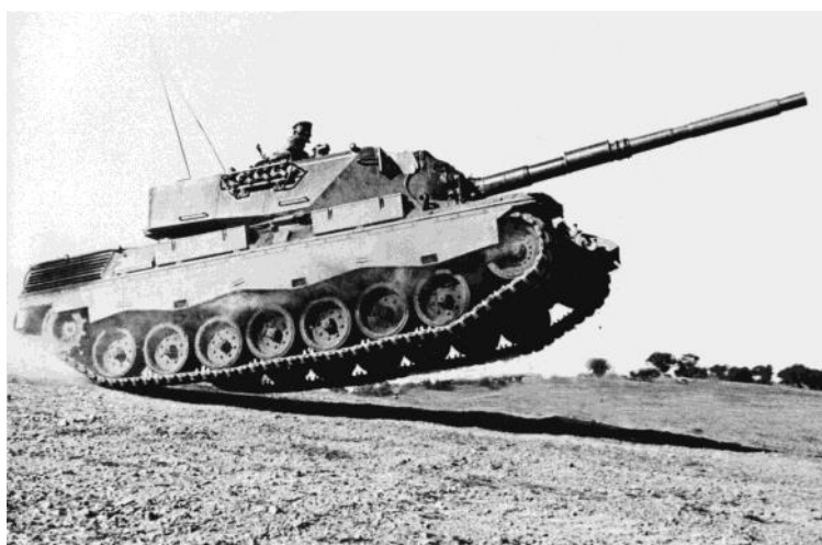
A leap forward in technology: a Leopard ASI MBT demonstrates its speed and power in a 'leaping Leopard' mobility display. Moving so quickly over the brow of a hill on the Puckapunyal Military Training Area, the Leopard leaves the ground momentarily before coming soundly back to earth, the impact handled by Leopard's torsion bar suspension. Although a crowd-thrilling feature of early displays, the 'leaping Leopard' was subsequently banned due to the wear and tear on suspension components. (School of Armour)
